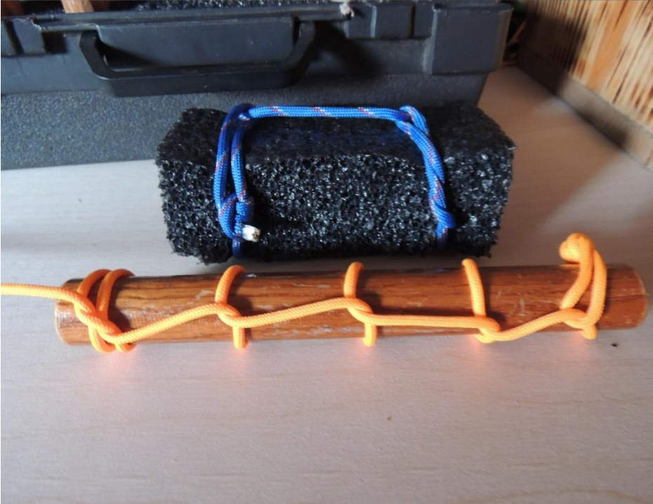
Half hitching using webbing with an overhand on a bight and a tautline hitch.
